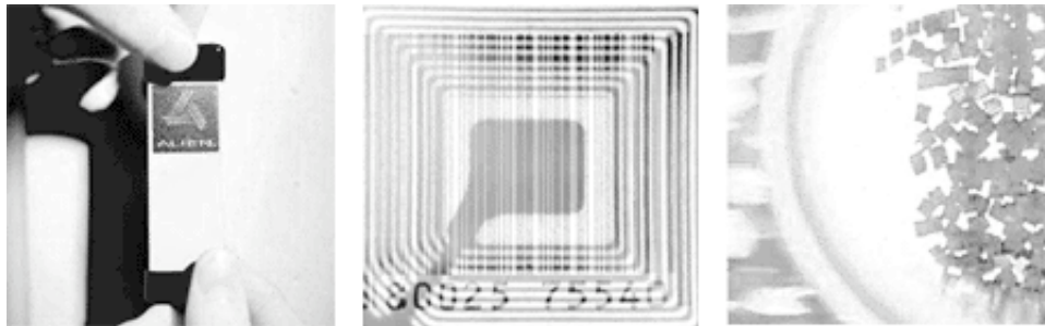
Fig. 1. A passive RFID tag, an RFID tag with a printed barcode, and dust-sized RFID microchips.
