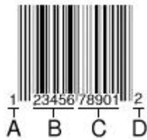
Figure 1-1: A standard UPC. Code components are labeled as follows: (A) Application Code (B) Manufacturer Code (C) Product Code (D) Checksum Digit
